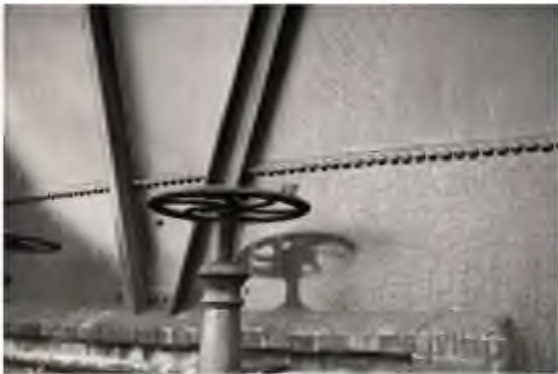
Figure 3.8 Shadow effect: Unidentified photographer, "shadow" of a hand valve wheel on the painted wall of a gas storage tank; radiant heat instantly burned paint where the heat rays were not obstructed, Hiroshima, October 14–November 26, 1945. (Courtesy of the International Center of Photography.)
